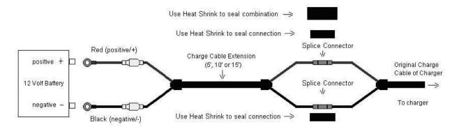
To connect the charger to the battery (batteries), route your charge cables from the charger to the batteries, being cautious to avoid sharp objects, and use the supplied wire ties to hold them securely and neatly in place.
